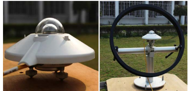
Fig. 4: Pyranometers with and without shadow ring for global and diffuse radiation measurements.
