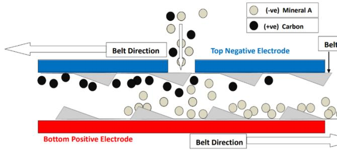
Fig. 9 Carbon particles charge positive in fresh ash processing of the Triboelectricstatic separation Method
