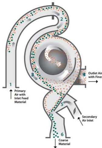
Fig.7 Diagram describing the centrifugal classifier technology
