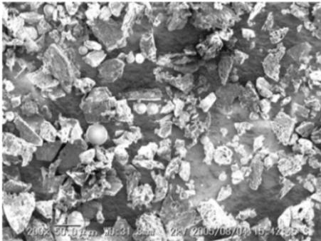
Fig. 5 the unburnt carbon after separation
