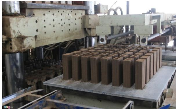
Fig. 6 The production of Aerated Autoclaved Concrete brick at the Song Da Cao Cuong Froth flotation factory in Viet Nam
