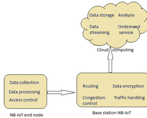
Fig. 1. Architecture of NB-IoT based HMS
