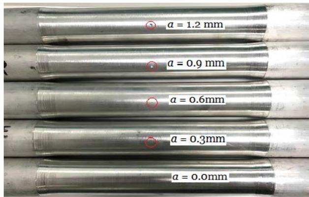
Fig. 8 A picture of local sharp-grooved 6061-T6 aluminum alloy tubes with  $D_o/t = 16.5$  and  $a = 0.0, 0.3, 0.6, 0.9$  and  $1.2$  mm.
