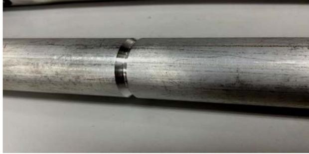
Fig. 1 A picture of the circumferential sharp-notched tube.
