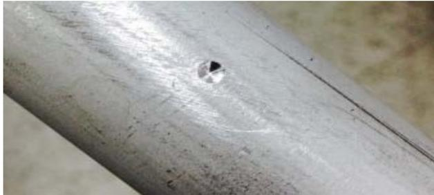
Fig. 3 A picture of the local sharp-notched (sharp-grooved) tube.
