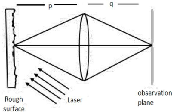
**Figure (3): scheme speckle pattern formation under illumination of a rough surface by laser light**
