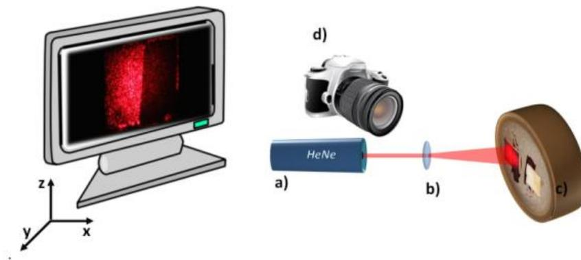
Figure (2) Schematic diagram of the experimental setup: (a) Laser HeNe wavelength 633nm; (b) focusing lens with  $f = 10\text{cm}$ ; (c) samples; (d) camera Canon T1. [12]
