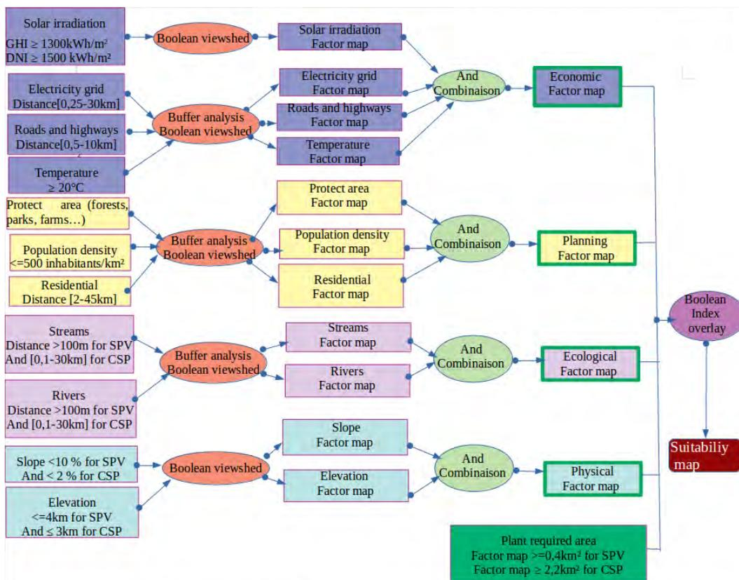
Fig.4: GIS based model solar SPV and CSP farm site selection
