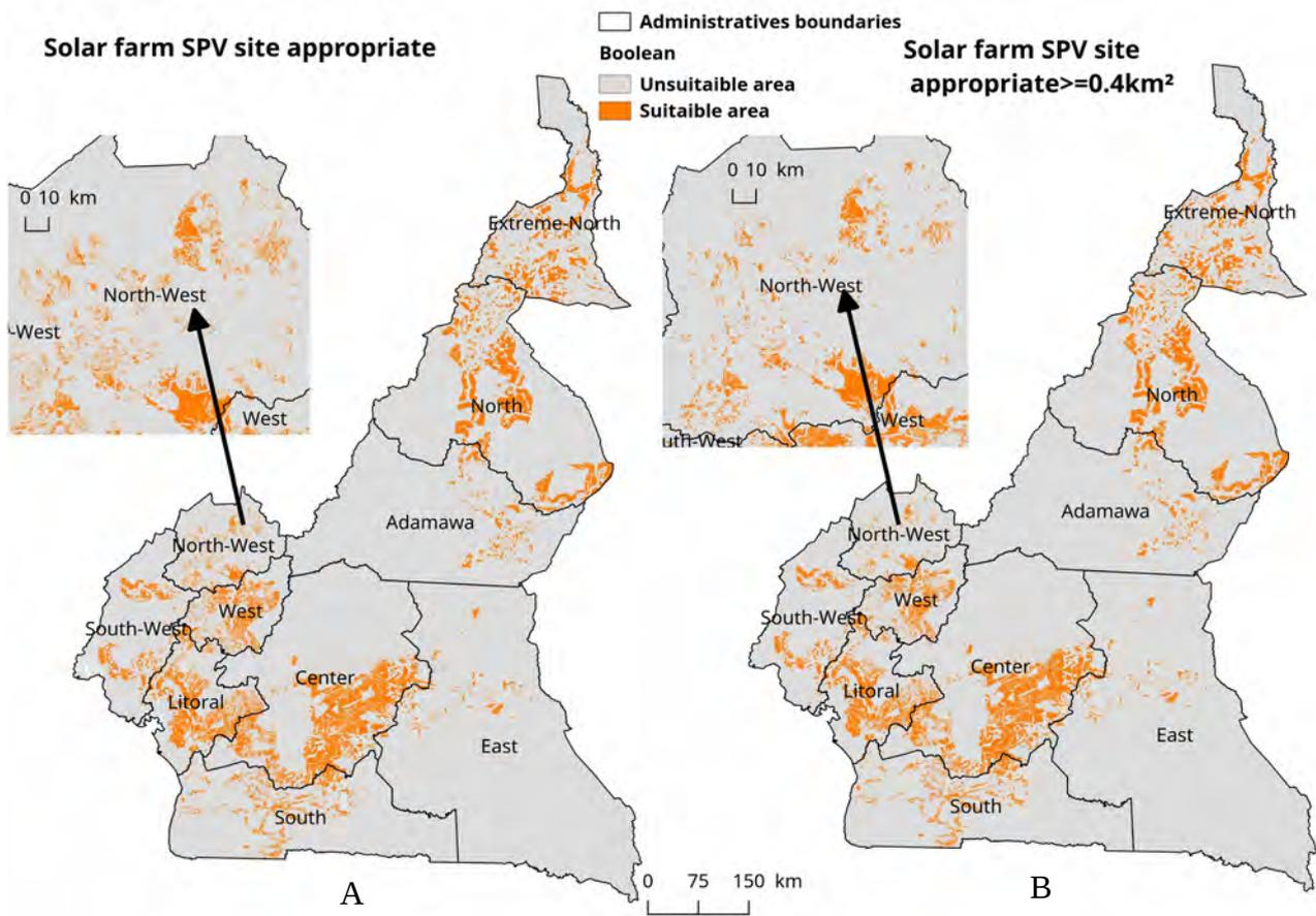
Fig.9: Suitability maps for Solar farm SPV (A) and Solar farm SPV  $\geq 0.4\text{km}^2$  (B)
