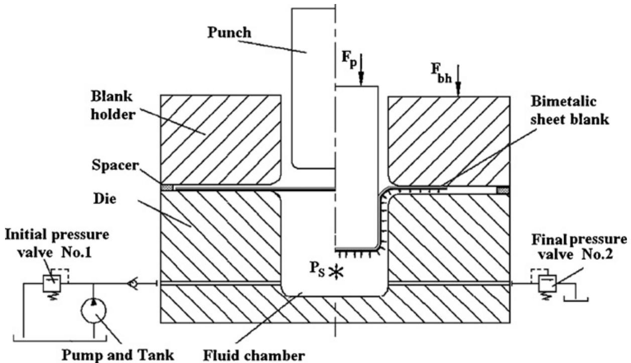
Fig 1.Hydro-deep drawing process of bimetal sheet
