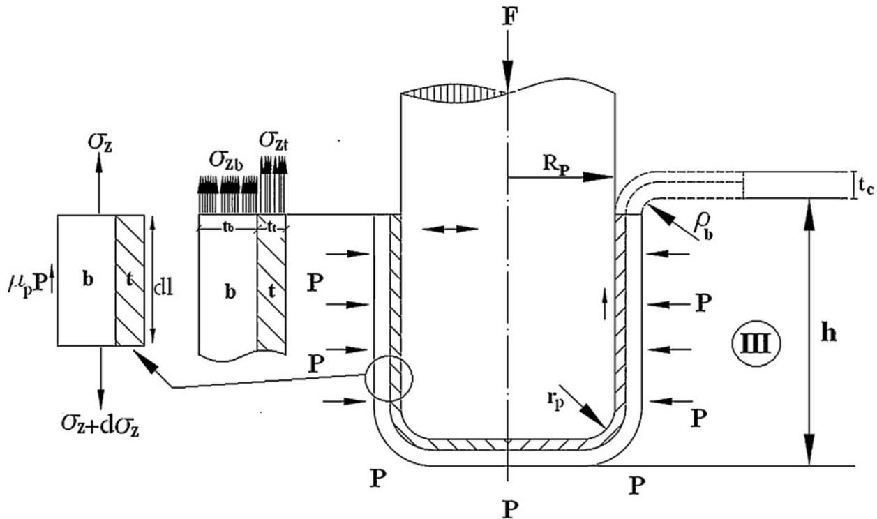
Fig 2. Bimetallic sheet in wall region equilibrium structure
