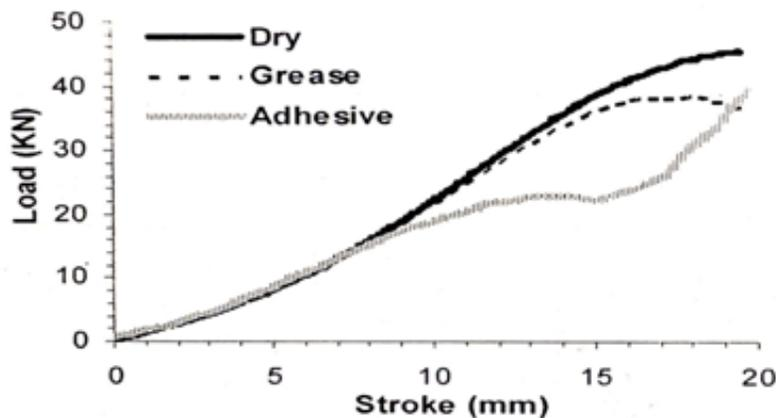
Fig 3. Contact condition effect on two layers in drawing process
