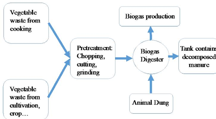
Fig. 1 Principle of a hybrid biogas system.
