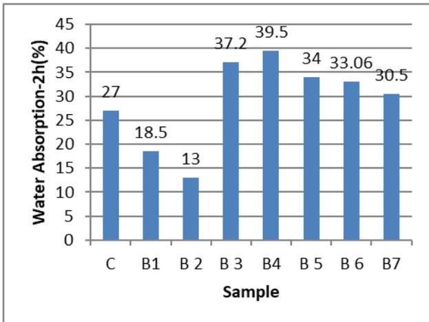
Fig-7 Water absorption (2h) property of light weight panels
