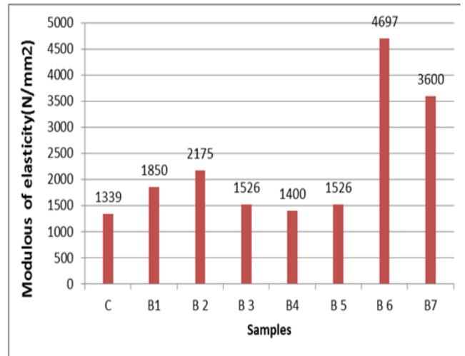
Fig-10 Modulus of Elasticity of light weight panels
