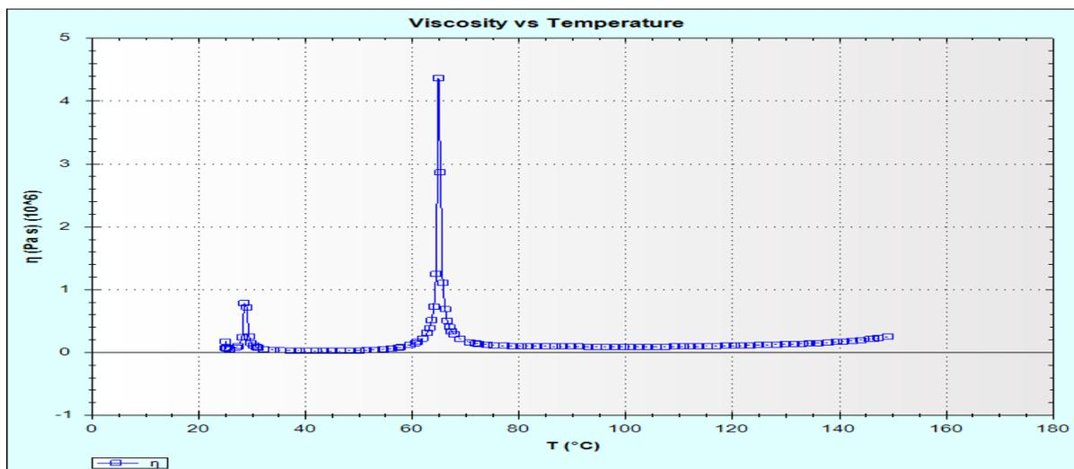
Fig.2. parallel plate viscosity of PF resin with 5% ammonium carbonate
