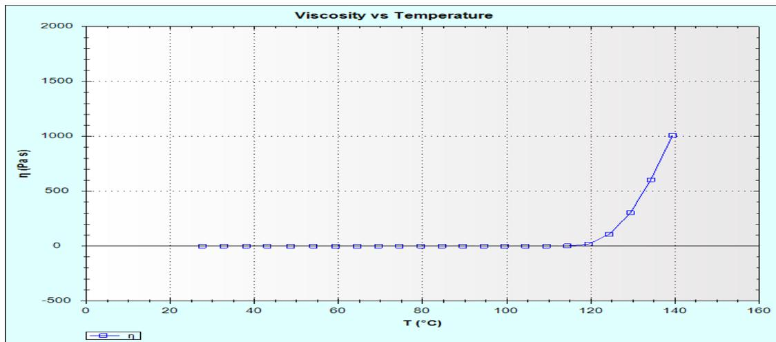
Fig.1. parallel plate viscosity of PF resin
