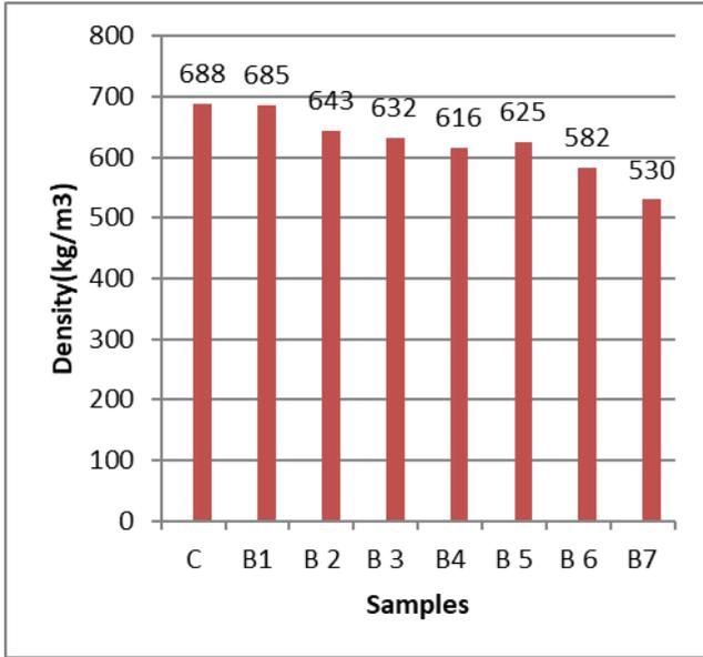
Fig-5 Density of light weight panels
