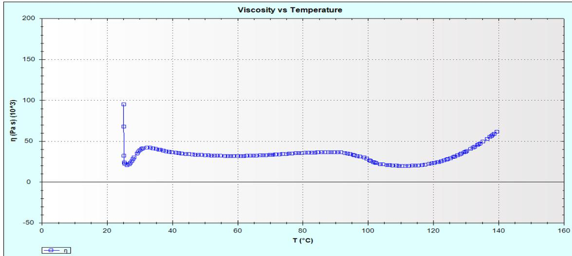
Fig.3. parallel plate viscosity of MUF resin
