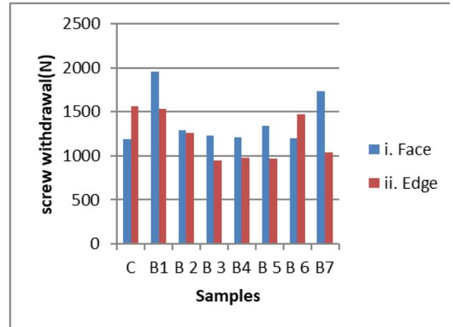
Fig- 12 Screw withdrawal property of light weight panels
