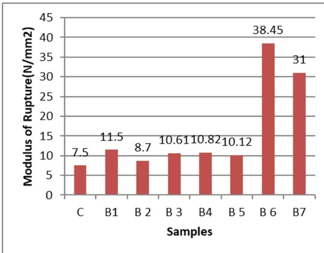
Fig-9 Modulus of Rupture of light weight panels
