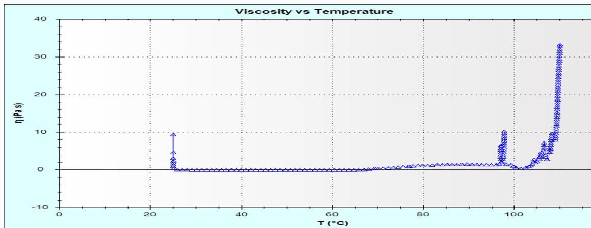
Fig-4. parallel plate viscosity of MUF resin with Ammonium carbonate
