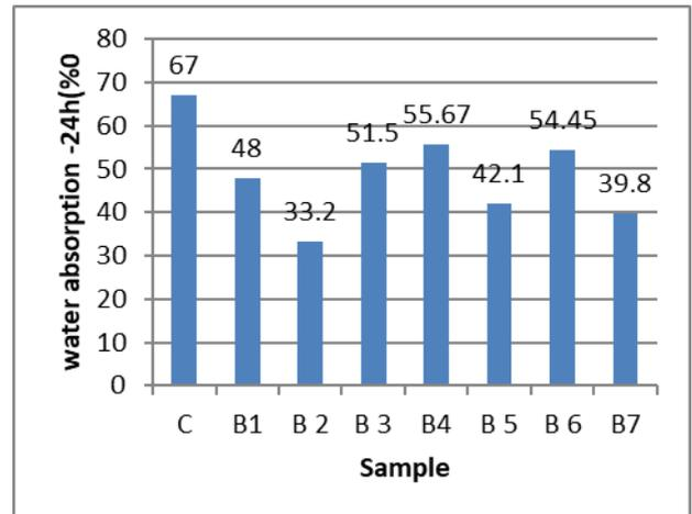
Fig-8 Water absorption (24h) property of light weight panels
