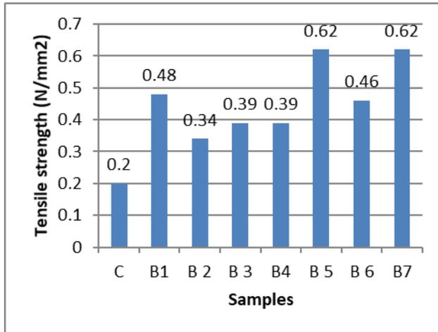
Fig- 11 Tensile strength property of light weight panels
