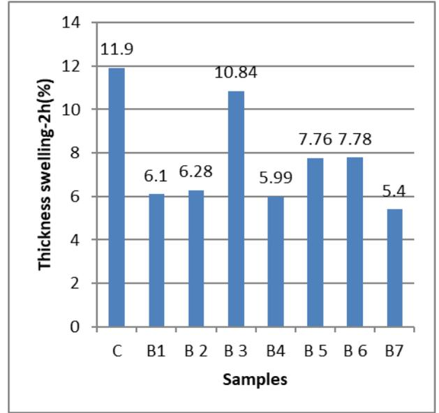
Fig-6 Thickness swelling properties of light weight panels
