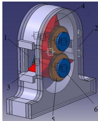
Fig. 2. Axonometric view of the volumetric rotating machine model with profiled rotors
