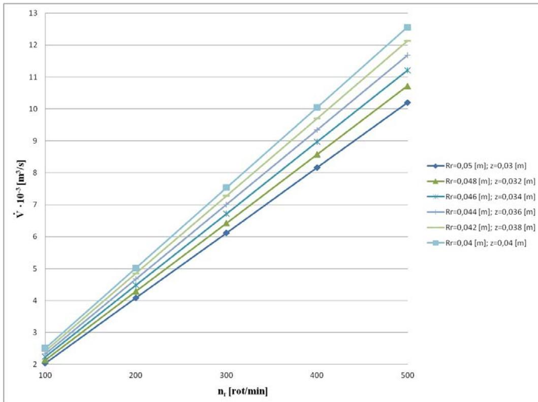
**Fig. 5.** Variation of volumetric flow rate according to  $n_r$ ,  $R_r$  and  $z$
