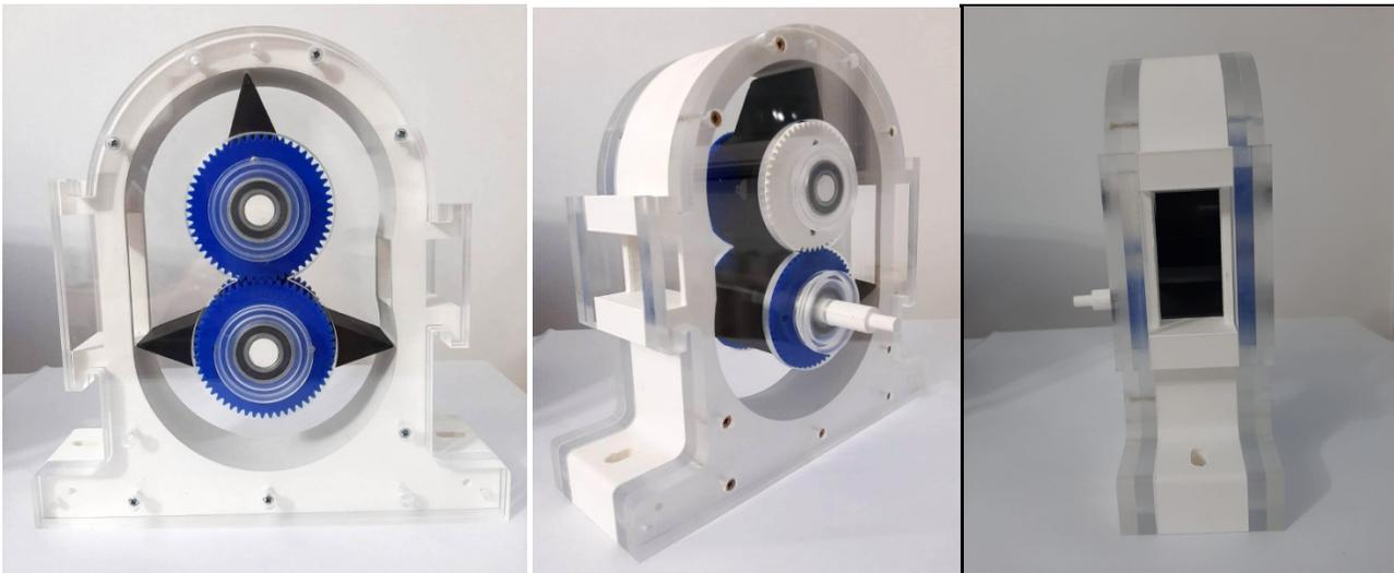
Fig. 6.. Longitudinal end transversal view of the model of the working machine
