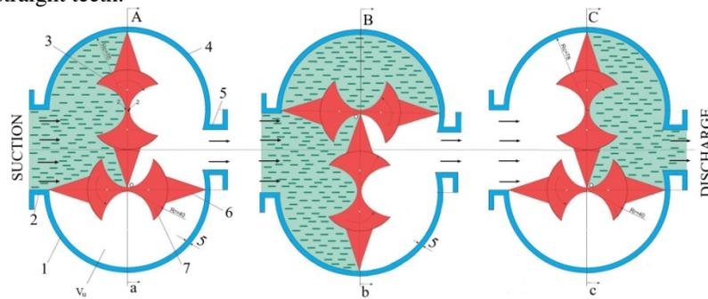
Fig. 1. Operating principle of the rotating volumetric machine
