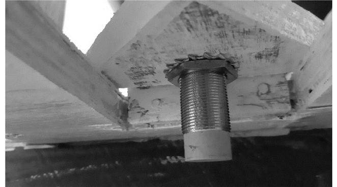
Fig. 6 Capacitive proximity sensor placement
