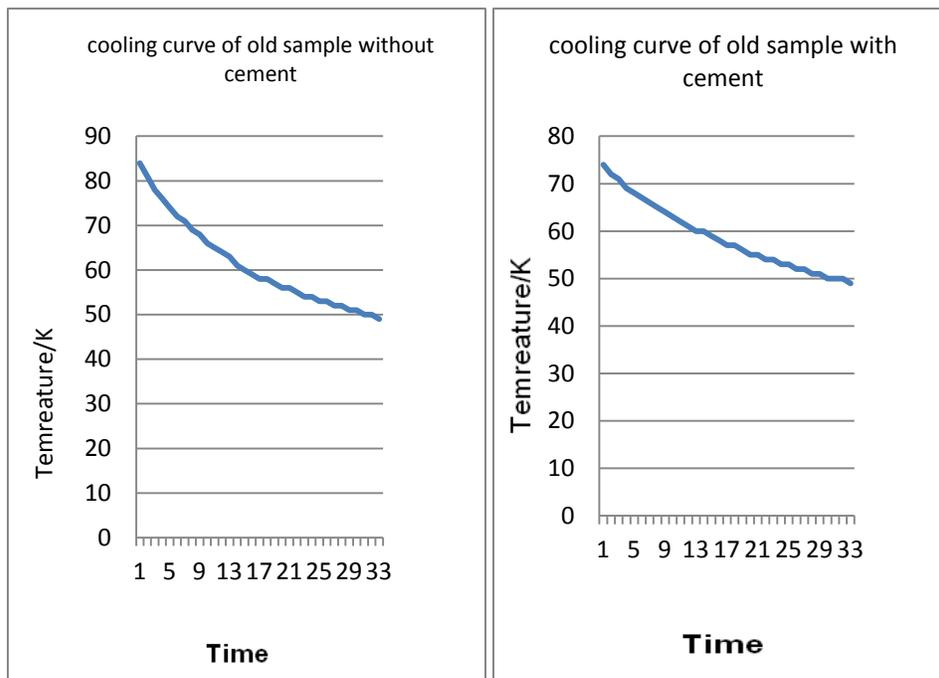
Figure3: Cooling curves of old sample with and without cement
