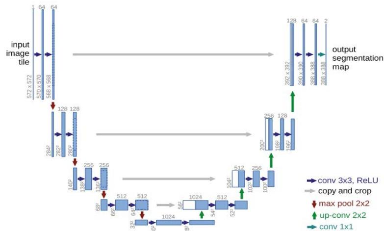
Fig. 1. Architecture of U-Net
