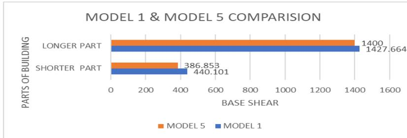
Fig 15 – comparison of base shear in model 1&5
