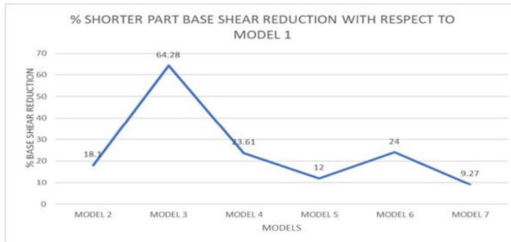
Fig. 19 – comparison % base shear reduction on shorter part of building of all models
