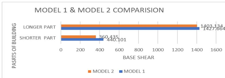
Fig. 12 – comparison of base shear in model 1&2
