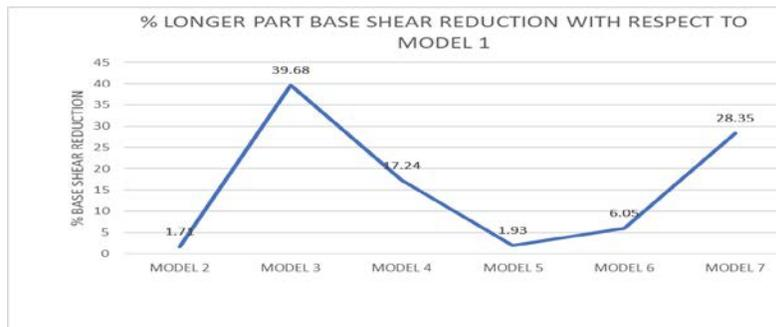
Fig. 20 – comparison % base shear reduction on longer part of building of all models
