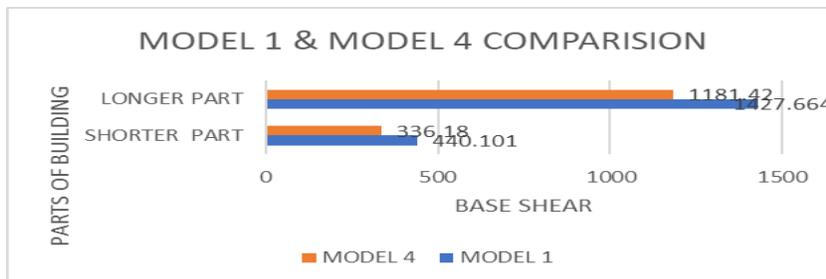
Fig. 14 – comparison of base shear in model 1&4
