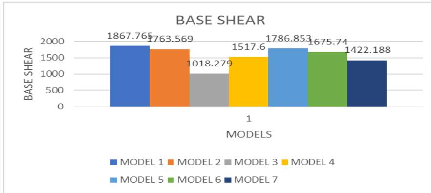
Fig. 18 – comparison of base shear in all models
