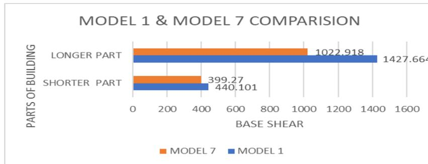
Fig 17 – comparison of base shear in model 1&7
