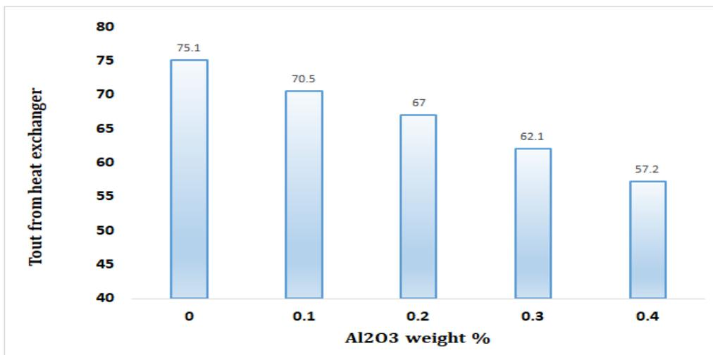
Fig. 10. Effect of Nano particle weight % at full load
