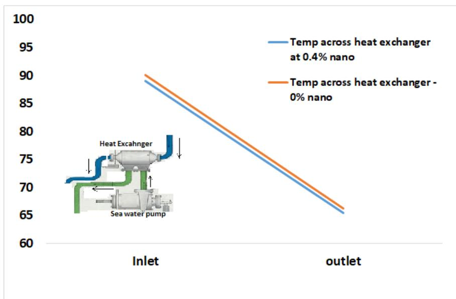
Fig. 7. Temperature across the heat exchanger for fresh water at no load
