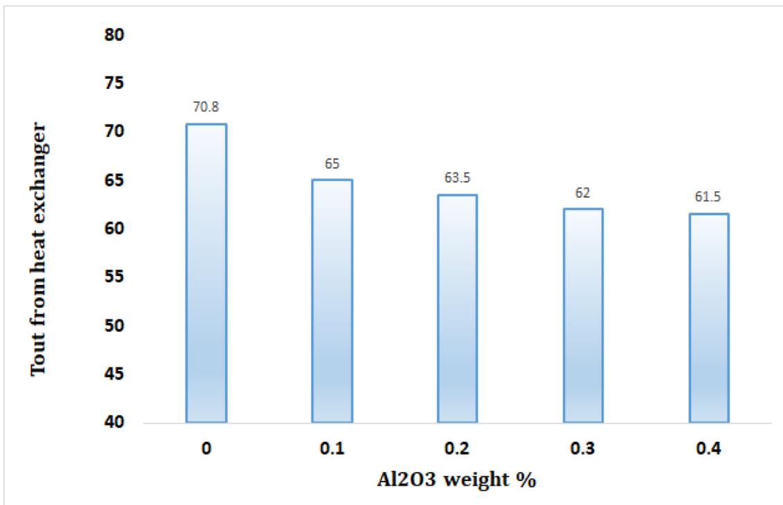
Fig. 8. Effect of Nano particle weight % at half load
