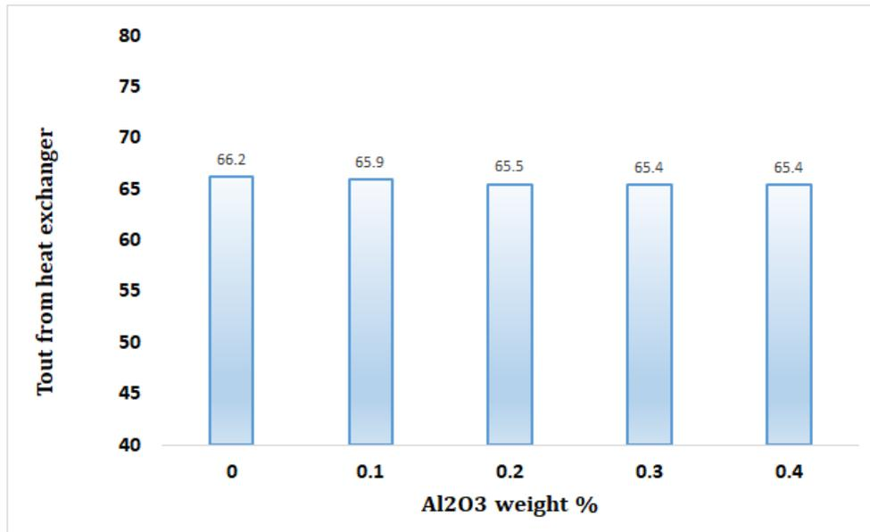
Fig. 6. Effect of nano particle weight % at no load
