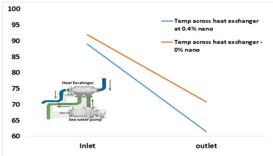
Fig. 9. Temperature across the heat exchanger for fresh water at half load
