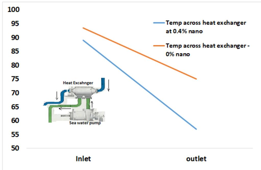
Fig. 11. Temperature across the heat exchanger for fresh water at full load
