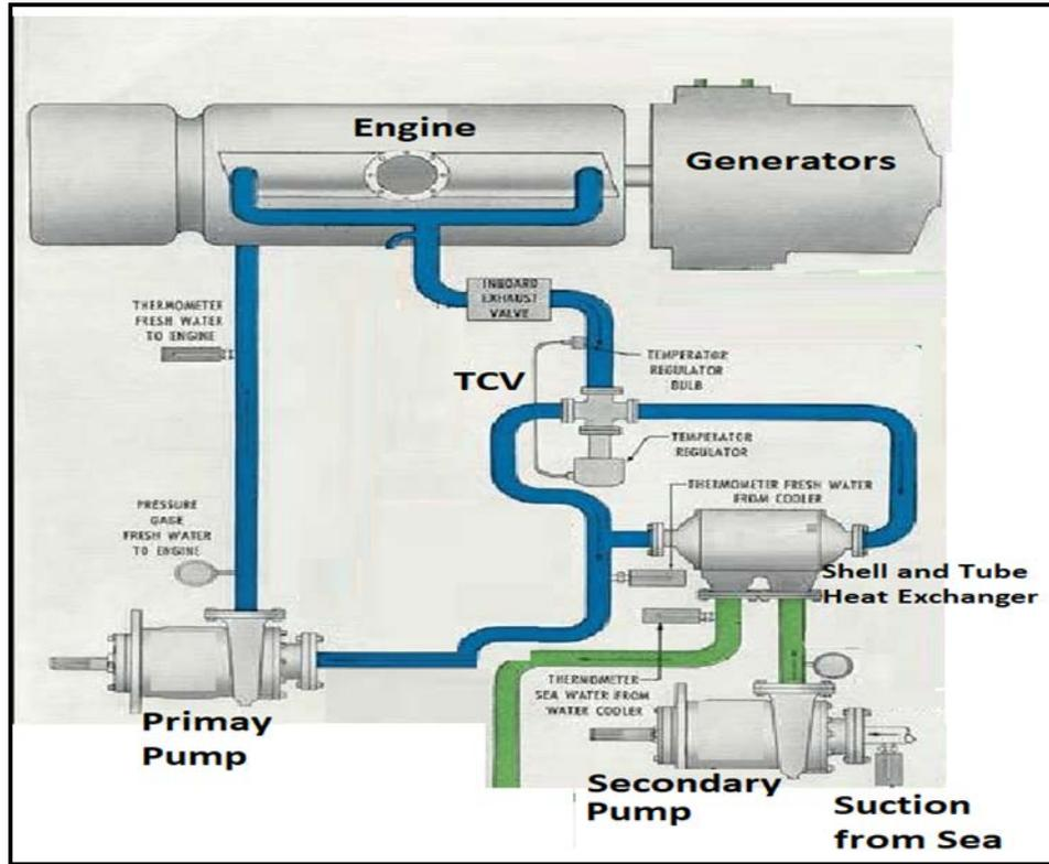
Fig. 4. Primary and secondary cooling cycle
