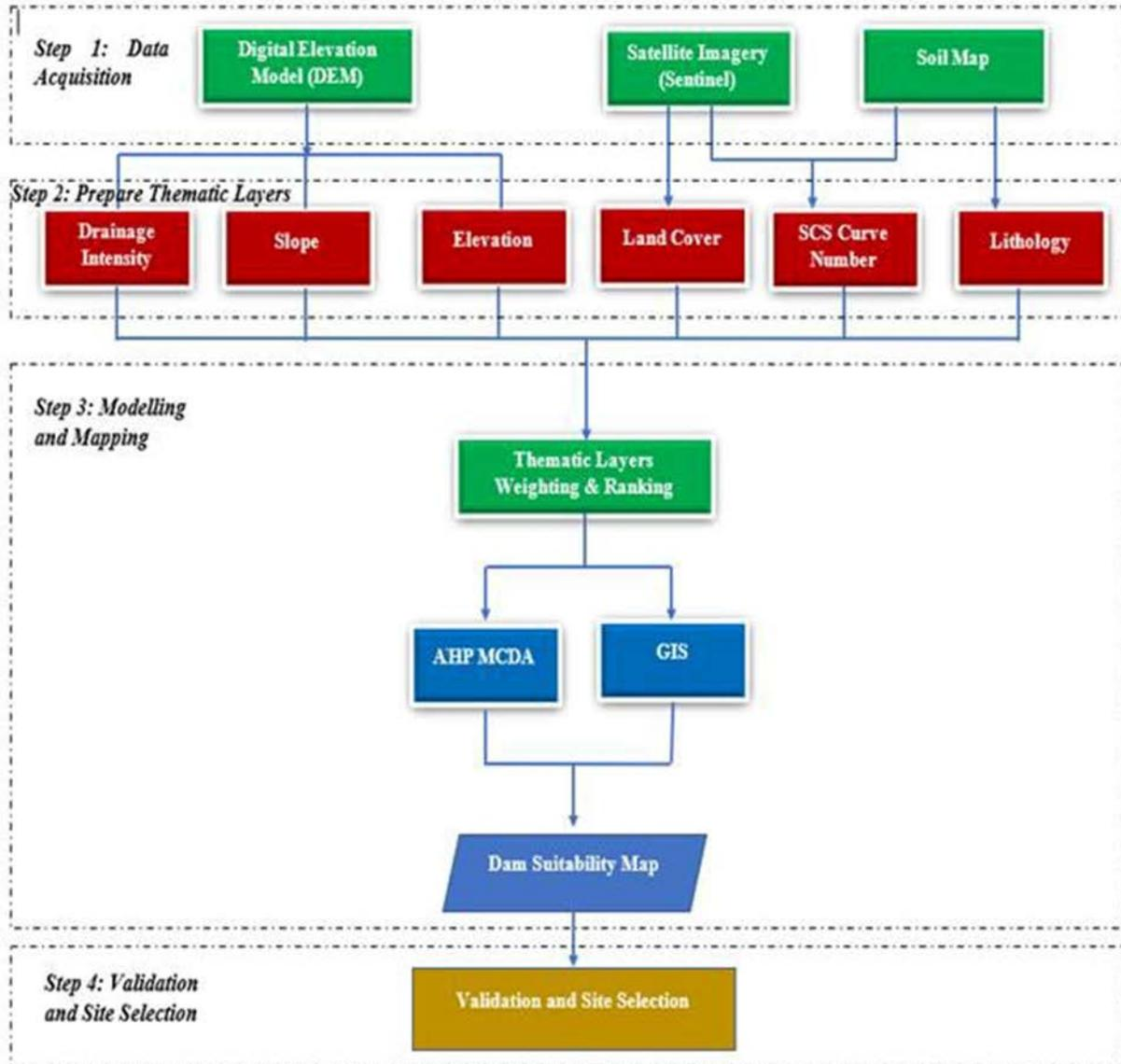
Figure 3: Step-by-step methodology selecting suitable sites for the dams. The approach is phased in four stages: Data Acquisition, Preparation of Thematic Layers, Modelling & Mapping, and Validation & Site Selection.
