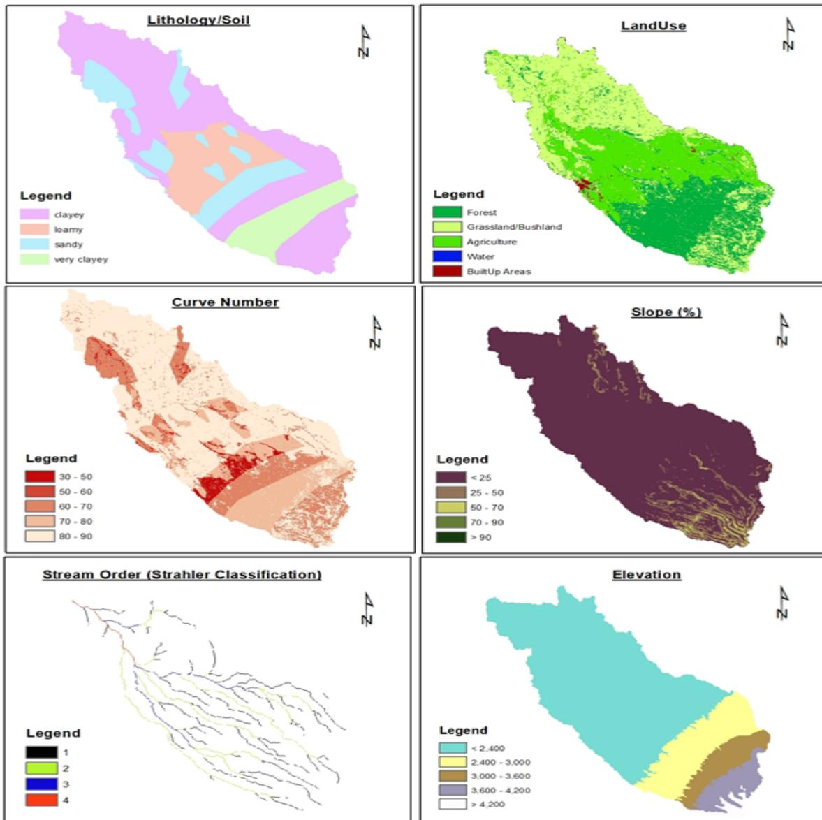
Figure 4: Maps of the thematic layers selected for AHP MCDA dam siting approach: Lithology and Soil, Land-use, curve number, slope, stream order and elevation.
