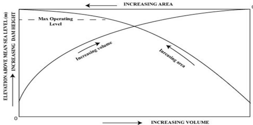
Figure 1: Typical reservoir elevation-area-volume relationship curve (AVE). The curve provides key design criteria and essential rules for reservoir operations (minimum and maximum operating reservoir level).
