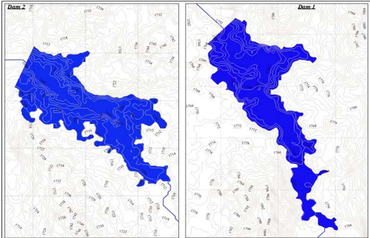
Figure 9: Illustration of the contours and the dams' top area at the two best selected locations. Note the numbers indicate the contour elevations.
