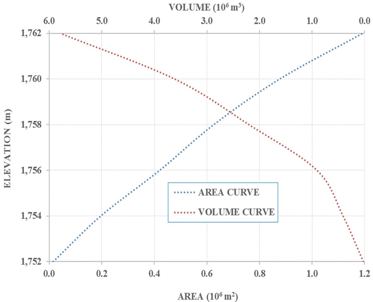
Figure 10: Elevation-Area-Volume Curve for the Proposed Dam No. 1
