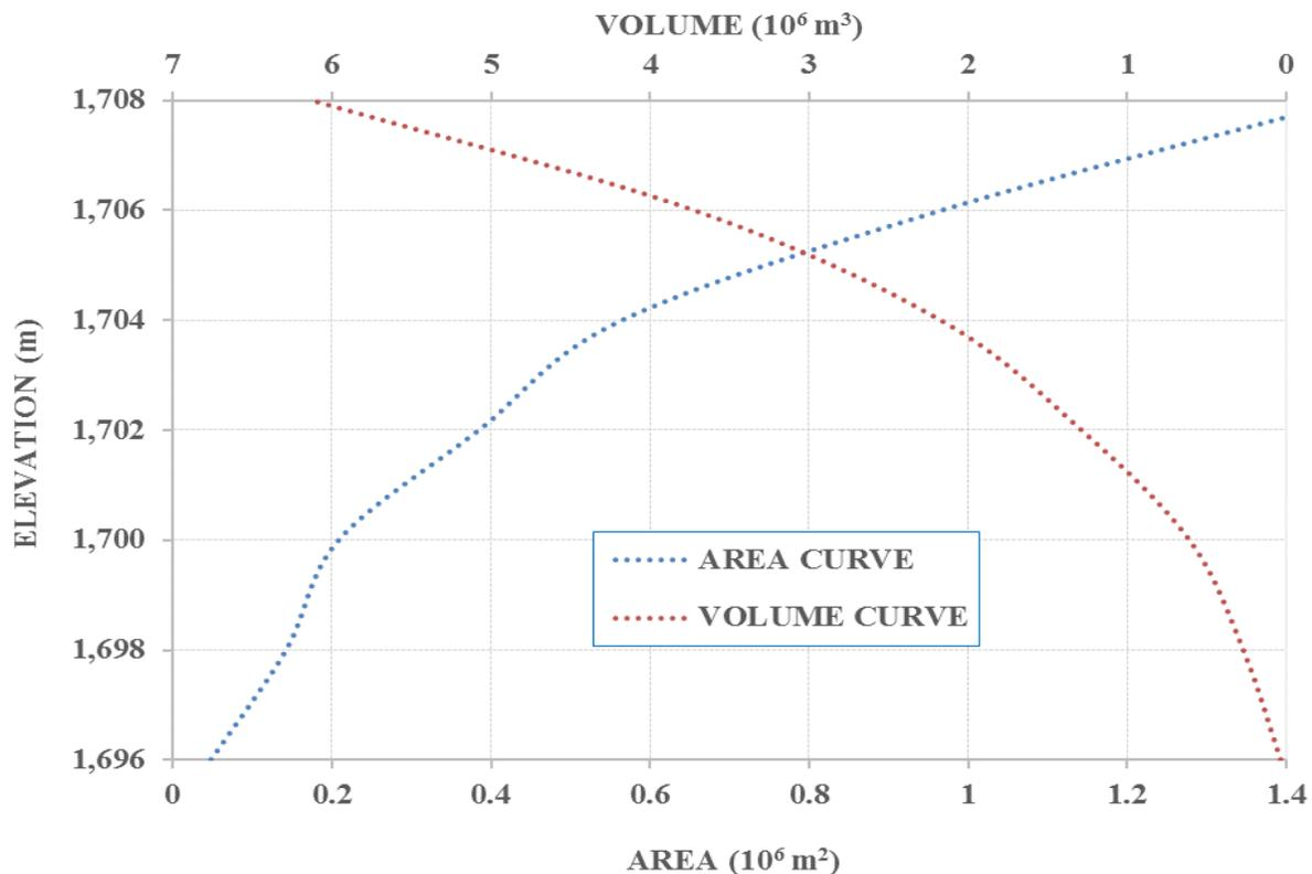
Figure 11: Elevation-Area-Volume Curve for the Proposed Dam No. 1
