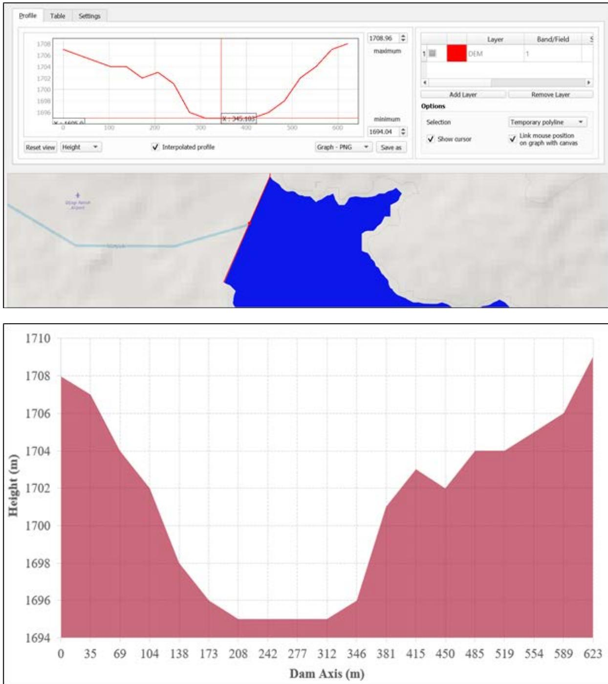
Figure 8: a) Profile of the Dam axis at dam location 2 extracted using the profile tool in QGIS from a Digital Elevation Model (DEM). b) Profile plot for dam 2 axis in excel.
