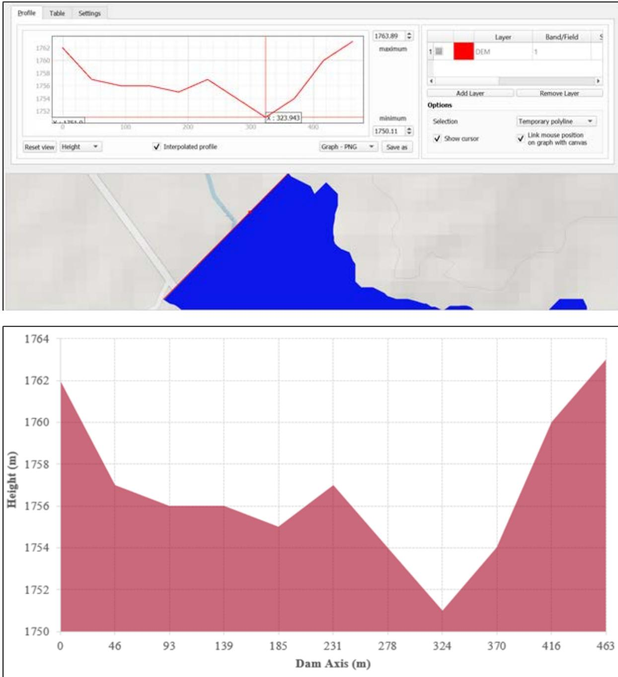
Figure 7: a) Profile of the Dam axis at dam location 1 extracted using the profile tool in QGIS from a Digital Elevation Model (DEM). b) Profile plot for dam 1 axis in excel.
