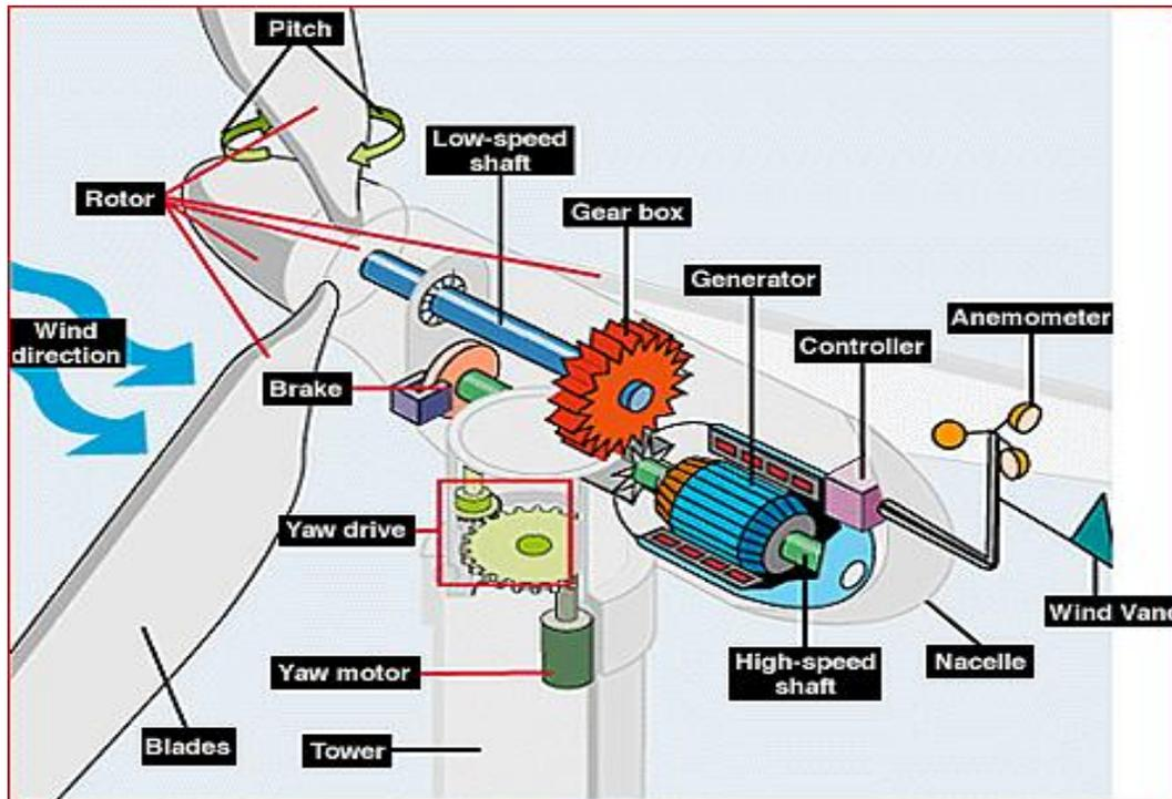
Fig. 2 Components of a wind turbine
