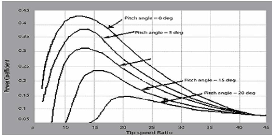
Fig. 4 Power Coefficient vs Tip speed ratio for various values of pitch angle
