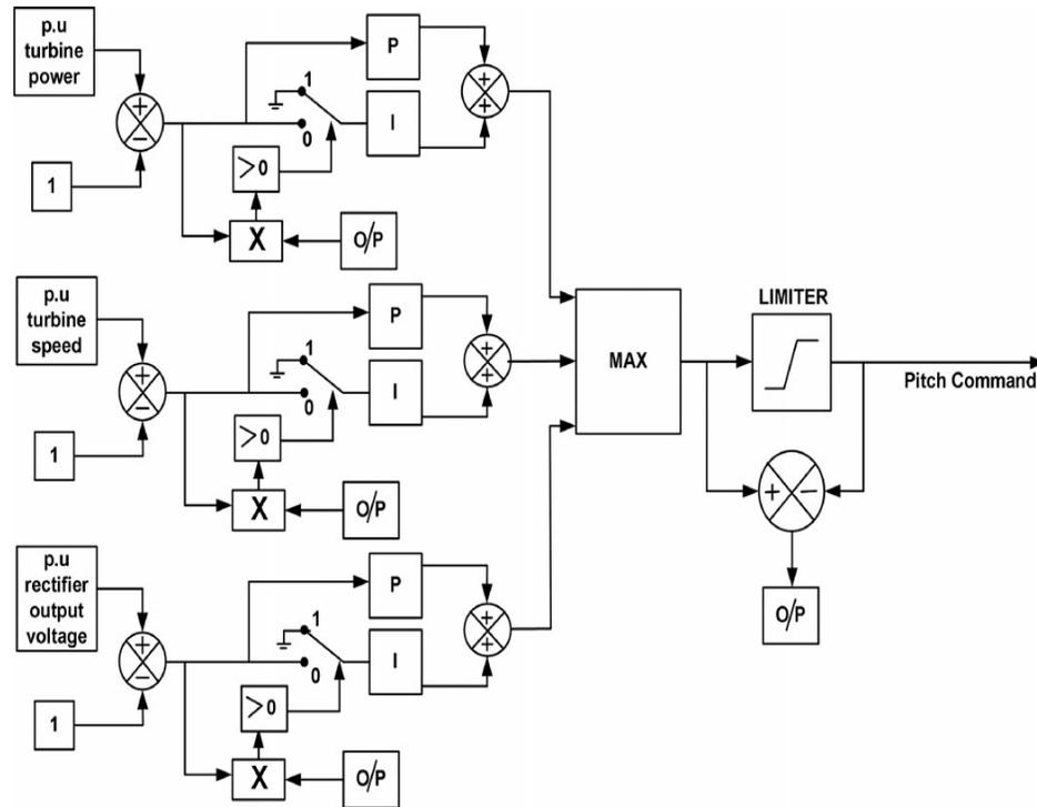
Fig. 7 Pitch control scheme for a stand-alone WECS
