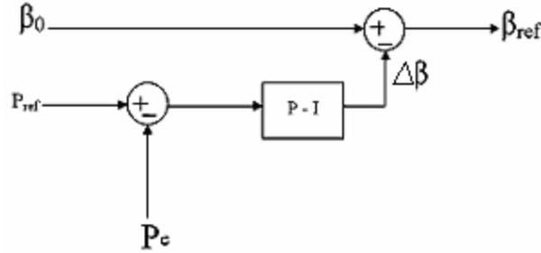
Fig. 6 Pitch angle reference generator
