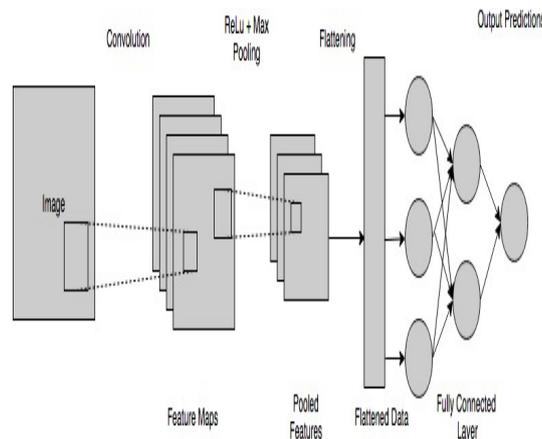
**Fig 3.3: Structure of Palm Print Detection.**
