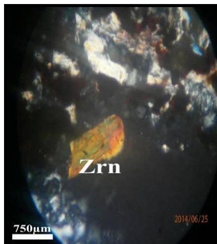
Fig.9: Photomicrograph showing short minute prismatic zircon (Zrn) crystals.
