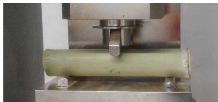
Figure 4: Three-point bending test on a bamboo specimen.
