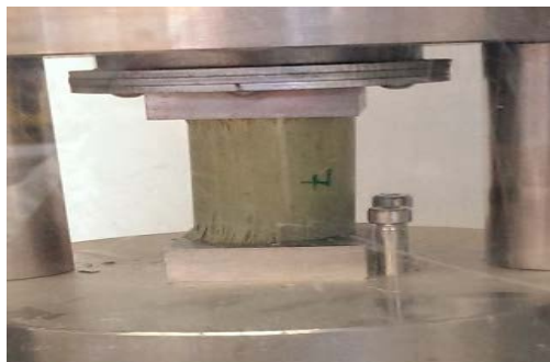
Figure 3: A bamboo specimen during the uniaxial compression test.
