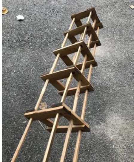
Figure 2: Details of bamboo reinforcement ( Nurharniza et al., (2022) ).
