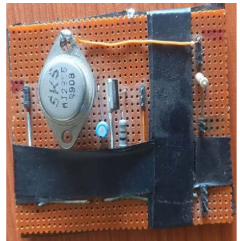
Figure 3: (a) Schematic circuit diagram of the 5 V power supply and (b) Pictorial view of the 5 V power supply circuit
