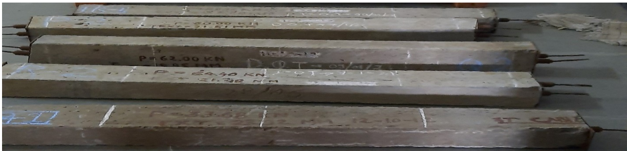
Fig 2: Prestressed concrete beams
