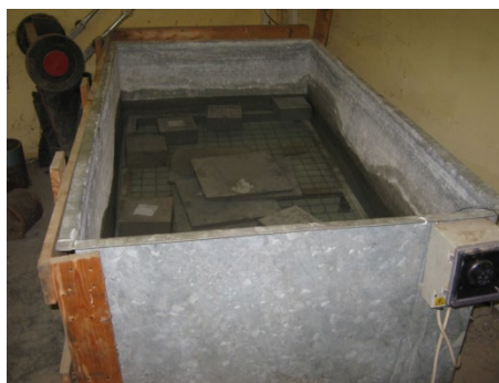
Fig. 1: Concrete cubes immersed in a water tank
