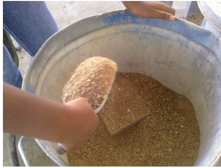
Fig. 2: Concrete cubes covered with wet sand in a bin
