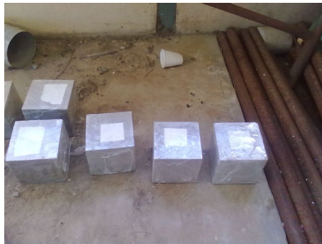
Fig. 3: Concrete cubes covered with plastic wrapping
