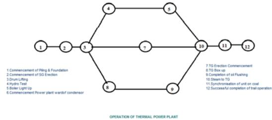
Fig. 1 Operational Thermal power plant PERT Network
