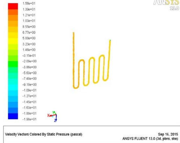
Fig.4.2. The Vector Pressure occurred on the water tube
