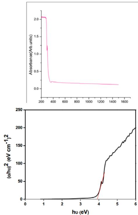
Fig 3 The Absorbance spectra & Band gap of as deposited ZnS thin film
