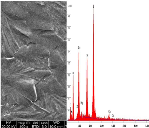
Fig 2 SEM Micrograph & EDAX of as prepared ZnS thin film
