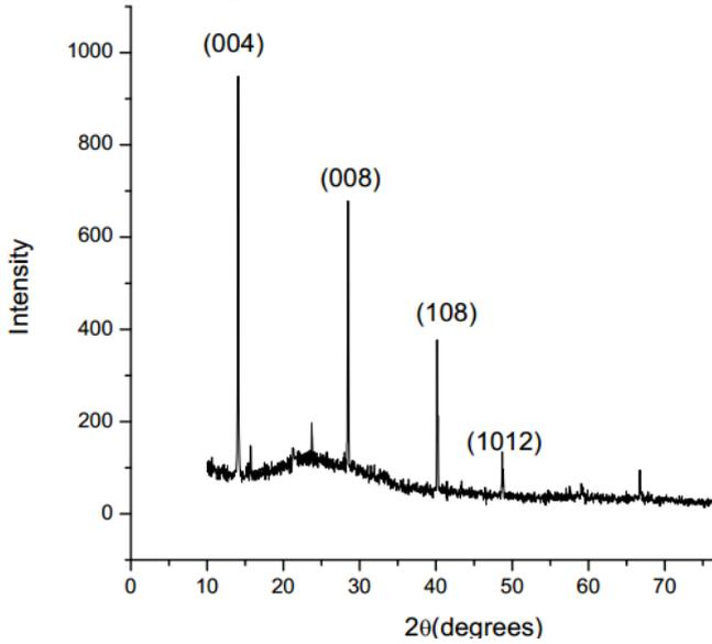
Fig 1. XRD Pattern of as prepared ZnS thin film
