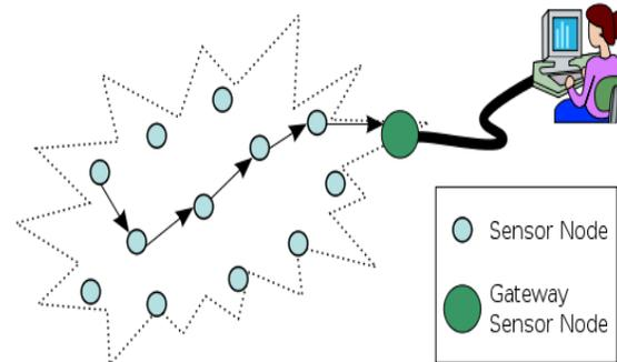
Figure1(a): Typical multi-hop wireless sensor network architecture
