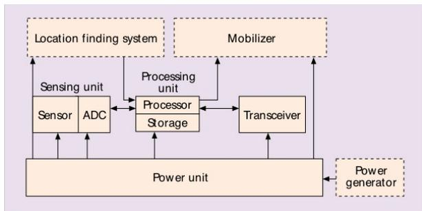
Figure 1. Structural view of sensor network [4]
