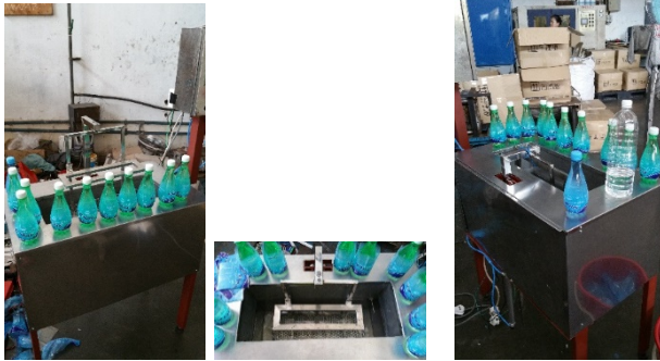
Appendix 2 Front view, top view and side view of the fabricated label shrinking machine.
