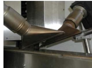
Fig. 2 Heat guns application
