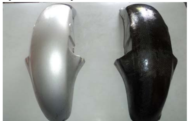
Fig. 2.5 Plastic & Carbon Fibre Mudguard
