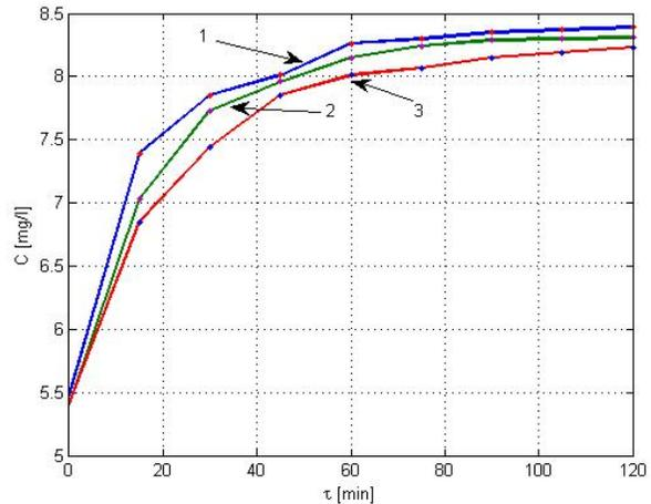
Fig. 11 The variation of dissolved oxygen concentration in water function of time
