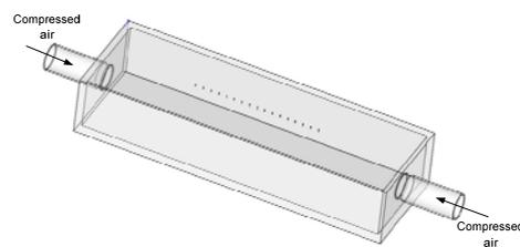
Fig. 6 Fine air bubble generator, version II.
