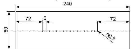
Fig. 5 Perforated plate with orifices of Ø 0.3 mm.
