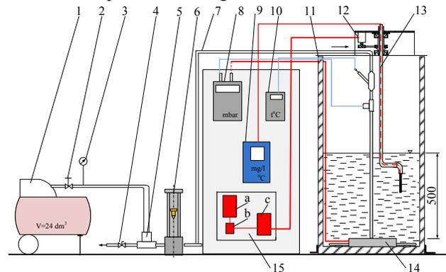
Fig. 10 Sketch of the experimental plant for researches regarding water oxygenation
