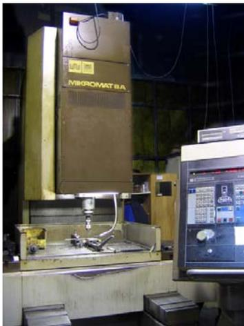
Fig. 9 Micro processing machine, Micromat type 6A.
