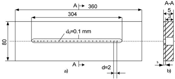
Fig. 1 The FBG perforated plate
