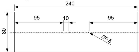
Fig. 7 Perforated plate with orifices of  $\varnothing 0.5$  mm.
