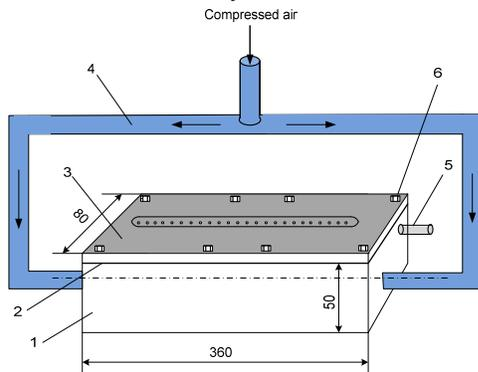
Fig. 2 Fine air bubble generator
