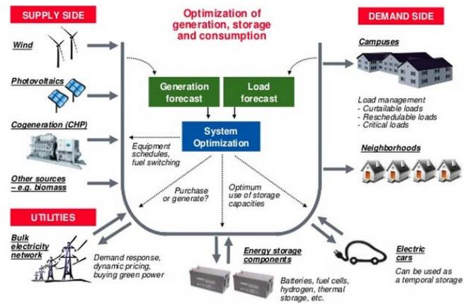
Fig.8. Integrated Intelligent Energy Management system
