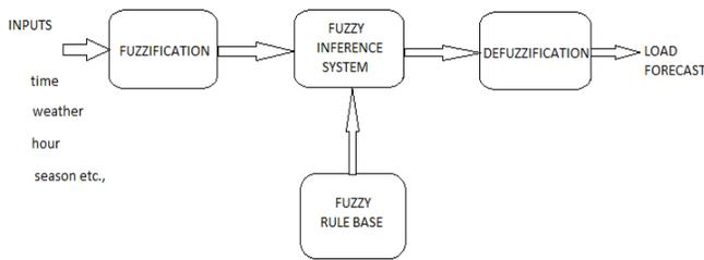
Fig.7. Fuzzy System for Load forecasting
