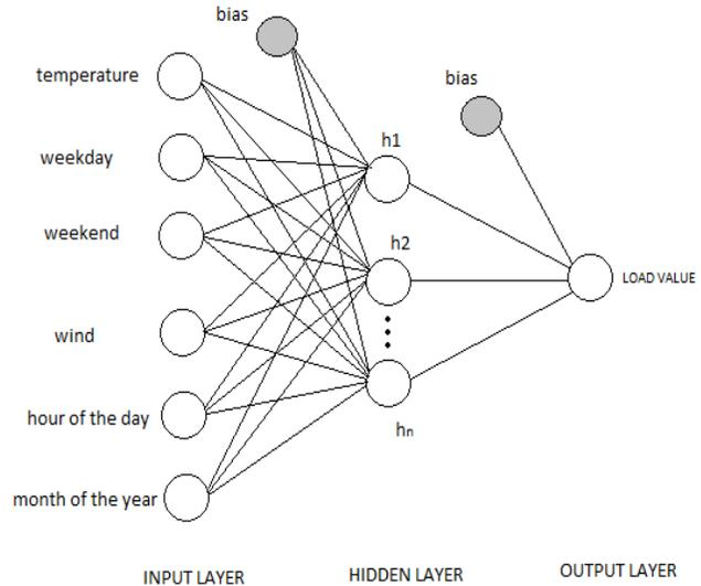
Fig. 6. Neural Network model for load forecasting
