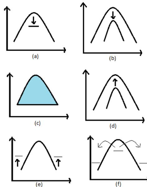
Fig.5. Demand side management – load shape objectives: (a) Peak clipping, (b) Conservation, (c) Flexible load shaping, (d) Load building, (e) Valley falling, (f) Load shifting
