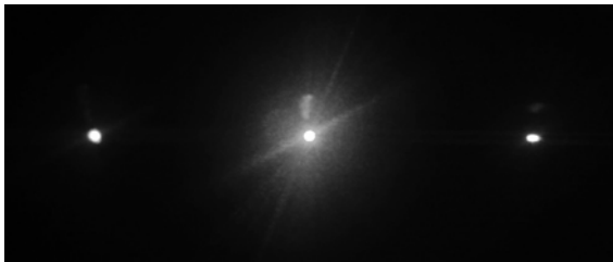
Figure 8(a): original compact disc which have 1600nm groove distance
