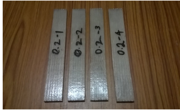
Fig. 5 specimen cut according to the ASTM standard D 7030
