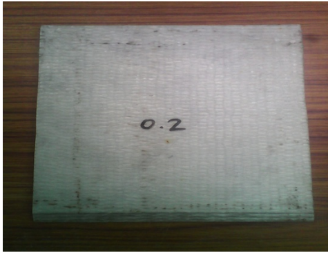
Fig. 4 GLARE laminate with 0.2 and 0.3 mm aluminium
