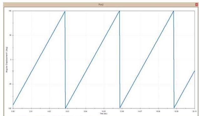
Graph 6.3 Angular displacement of crank
