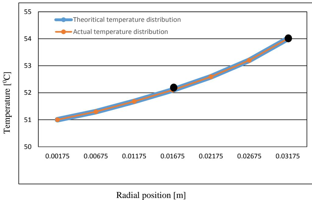
**Figure: 3** Temperature distributions in radial direction for the validation of radial heat transfer. The two black circles indicates the radial locations of two thermocouples
