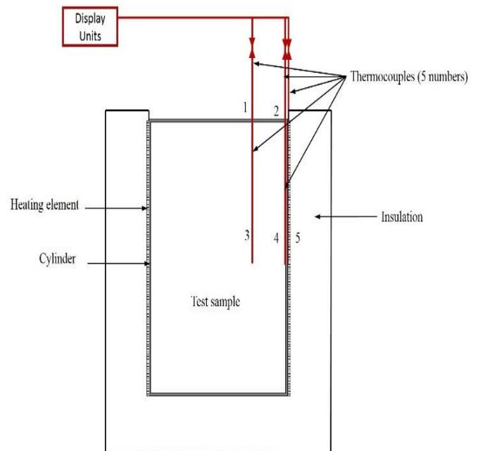
**Figure:1 Schematic diagram of experimental setup. (Locations of thermocouples are shown by numeric numbers)**
