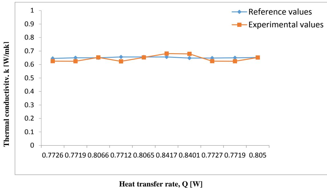
**Figure 4: Results of repeatability measurement of thermal conductivity for distilled water**
