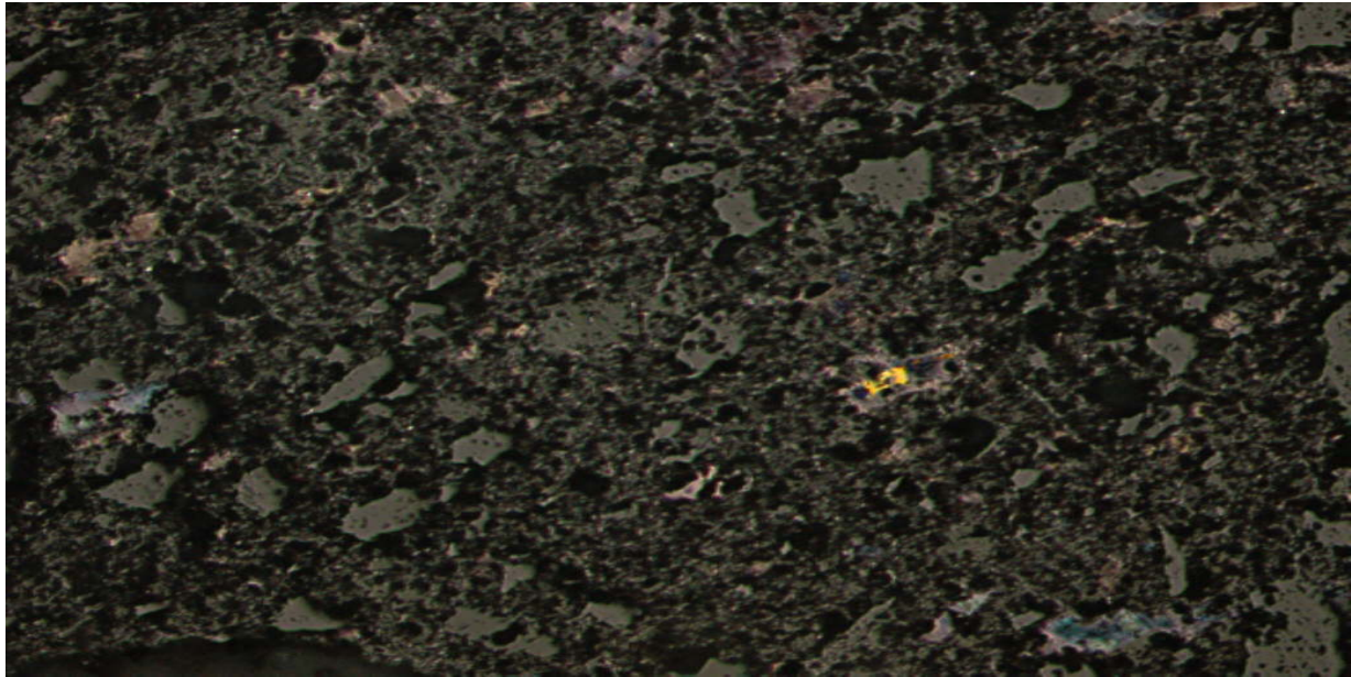
Figure 6: polished section Y02 with yellow crystal of chalcopyrite
