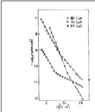
**Fig. 1** – Variation of dc-conductivity (-log  $\sigma$ ) versus 1/T, for the pellets of different composition of CuO-Bi<sub>2</sub>-O<sub>3</sub>
