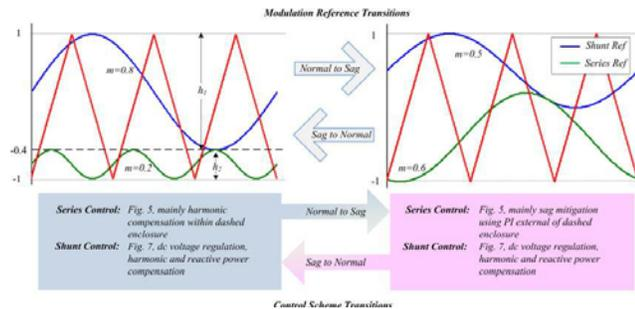
Fig.2.2 Transitions Of Modulating References And Control Schemes Between Normal (Left) And Sag Mitigation (Right) Modes.
