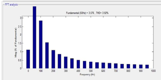
Fig 3.6: Total Harmonic Distortion of Source current shows 3.92% with PI controlled converter
