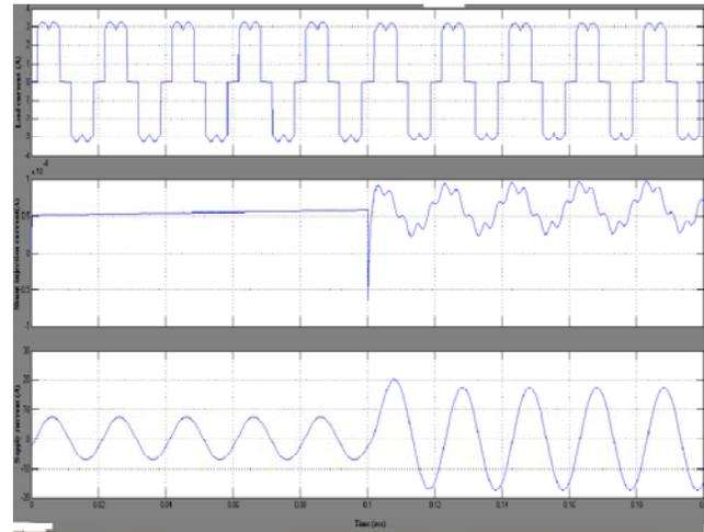
Fig. 3.9 Load, Shunt Injection and Supply Current during Normal to Sag Mode
