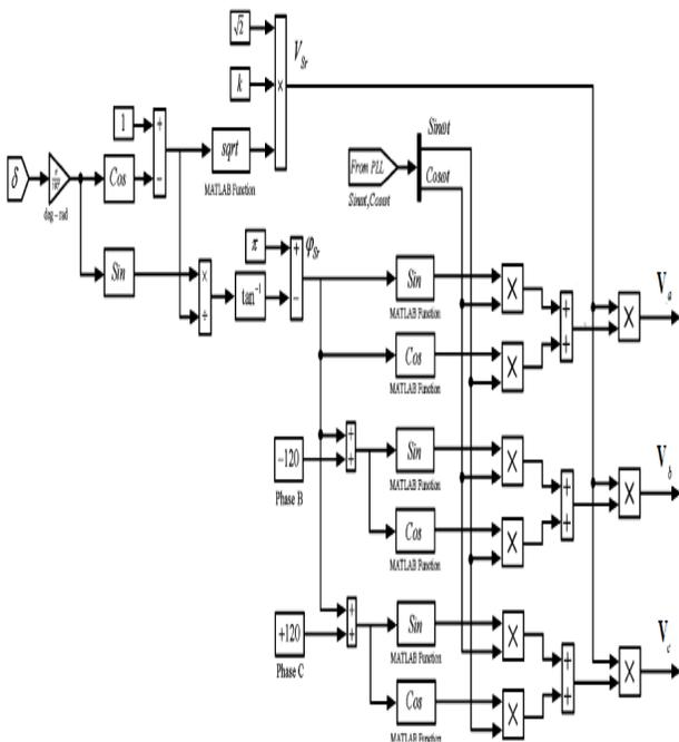
Fig. 3.3 Reference Signal Generation
