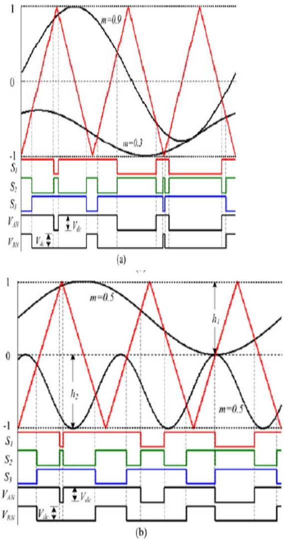
Fig. 2.1. Arrangements of reference having (a) the same frequency but different amplitudes, and (b) different frequencies but the same amplitude.
