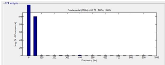
Fig 3.7: Total Harmonic Distortion of Source current shows 1.86% with Fuzzy controlled converter.
