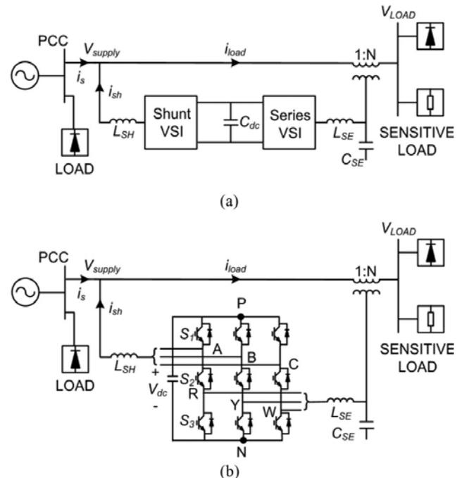
Fig. 1.Representations of (a) back-to-back and (b) nine-switch powerconditioners.
