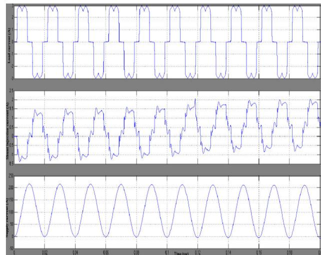
Fig. 3.5 Load, Shunt Injection, and Supply Current during Normal Power
