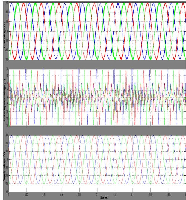
Fig. 3.4 Load, Series Injection, and Supply Voltages during Normal Power Conditioning Mode
