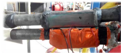
Figure 4 : TEGs sandwiched in between two ducts
