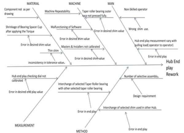
From the analysis of all the possible causes, three probable root causes are responsible for Hub End play rework in Rear axle assembly shop.
