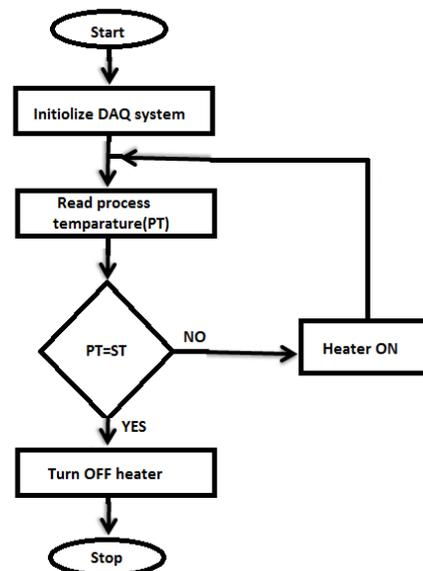
Figure-2 The flow chart for the system
