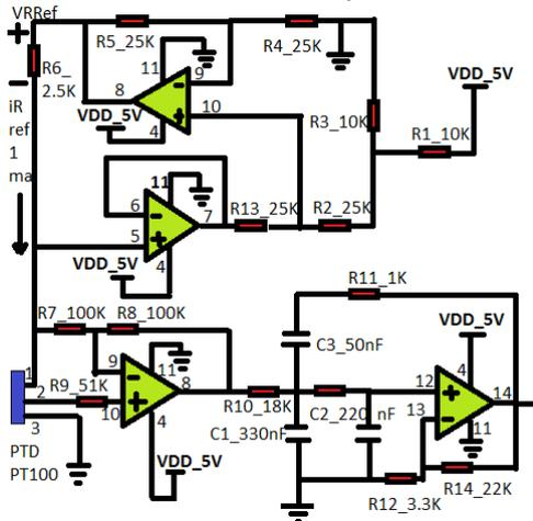
Figure-3 shows the PT100 sensor circuitry
