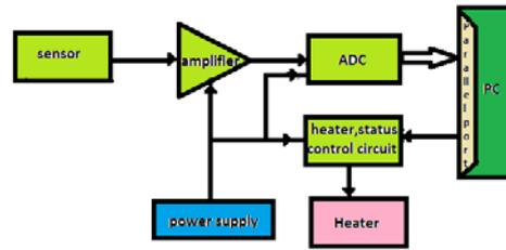
Figure-1 The block diagram of the Design of PC-based system for monitoring and control of a thermal process using LabVIEW.
