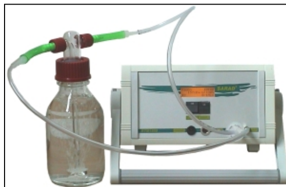
Figure 2. Concentration of ^{222}\text{Rn} measurement by Radon meter device RTM1688-2 model
