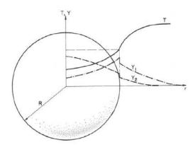
Temperature distribution of an evaporating liquid droplet
