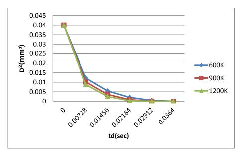
As the droplet lifetime increases diesel droplet get evaporates and burns. As the inlet atmospheric temperature is more it will evaporates and burns faster. From the above graph it shows that as compare to 600K and 900K , 1200K inlet temperature of air will evaporates faster. It satisfied the  $D^2$  – law of heat evaporation.
