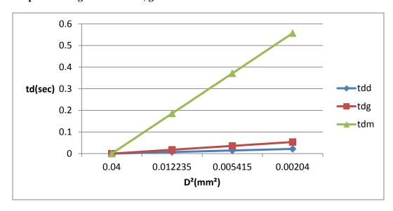
This graph shows diesel fuel evaporates faster than gasoline and ethanol. Because the boiling point and latent heat of vaporization or heat of combustion of diesel is more as compare to gasoline and methanol
