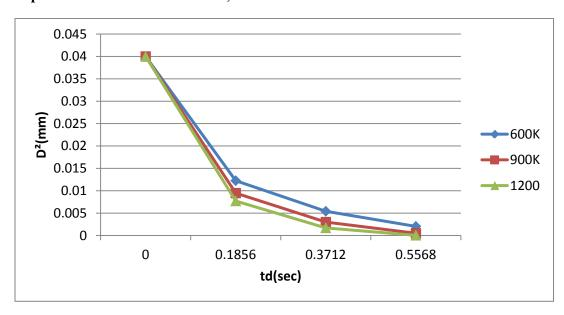
Above graph satisfied the  $D^2$  – law nature of graph is same as that of petrol and diesel but time required for the evaporation of droplet is more as compare to petrol and diesel. This is because of thermo physical properties of methanol.
