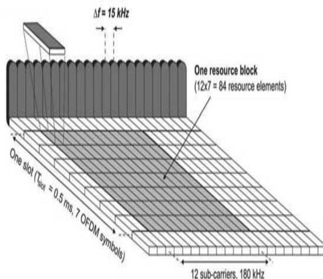
**FIGURE 1: LTE downlink physical resource based on OFDM**
