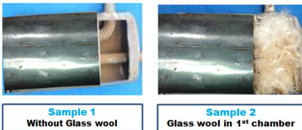
Fig. 6 Muffler sample with and without glass wool.
