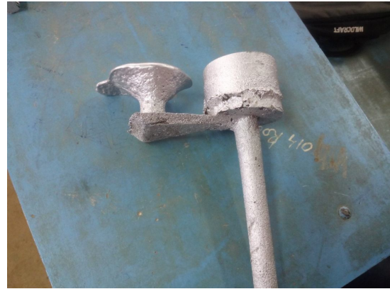
Figure 7. Test bar with gating system
