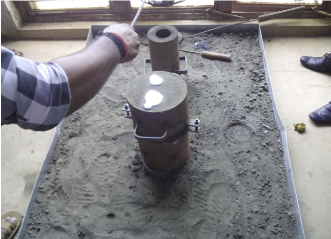
Figure 5. Pouring of molten metal to the mould
