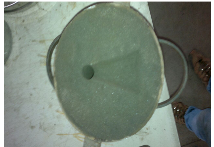
Figure 3. Moulding flask with groove for runner
