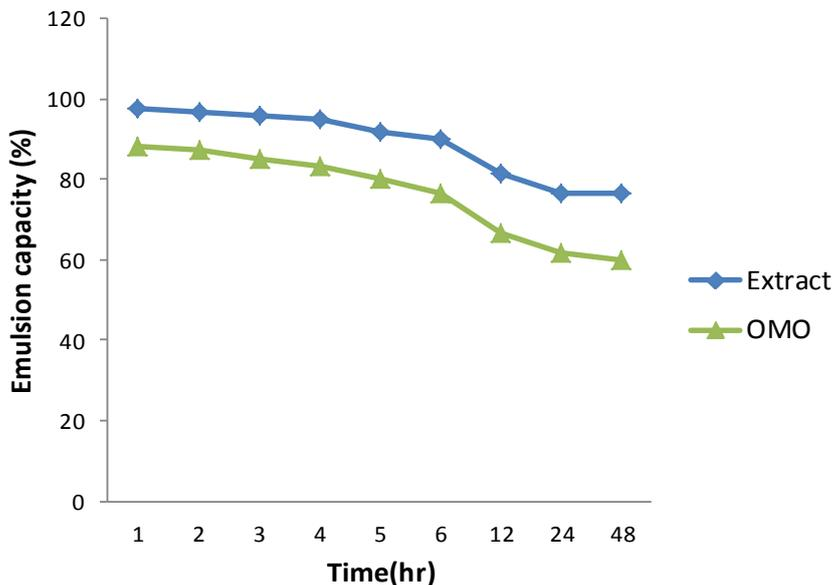
Figure 3: Emulsion Capacity (%) versus time (hr) for 2 g of Extracted Saponin-based surfactant and OMO Solutions.
