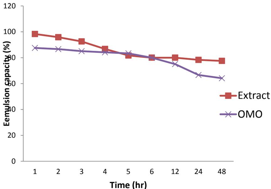
Figure 4: Emulsion capacity (%) versus time (hr) for 4 g of Saponin-based surfactant and OMO solutions.
