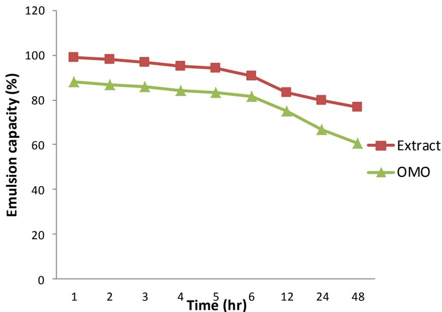
Figure 2: Emulsion capacity (%) versus time (hr) for 1 g of extracted Saponin-based surfactant and OMO solutions.
