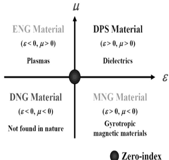
**Figure 1:** Different Types of Materials based on the values of Complex ( $\epsilon$ ) and ( $\mu$ ). Metamaterials can be divided into different categories by their two important parameters i.e. complex values of both the permittivity and permeability. Figure 1 helps to identify the various kinds of metamaterial structures. If permittivity ( $\epsilon_r$ ) and permeability ( $\mu_r$ ) are real and
