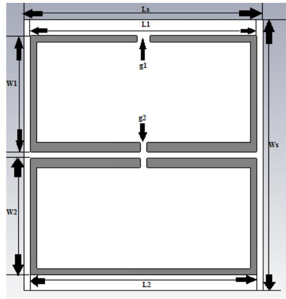
Figure 2 Front view of DNG Metamaterial
