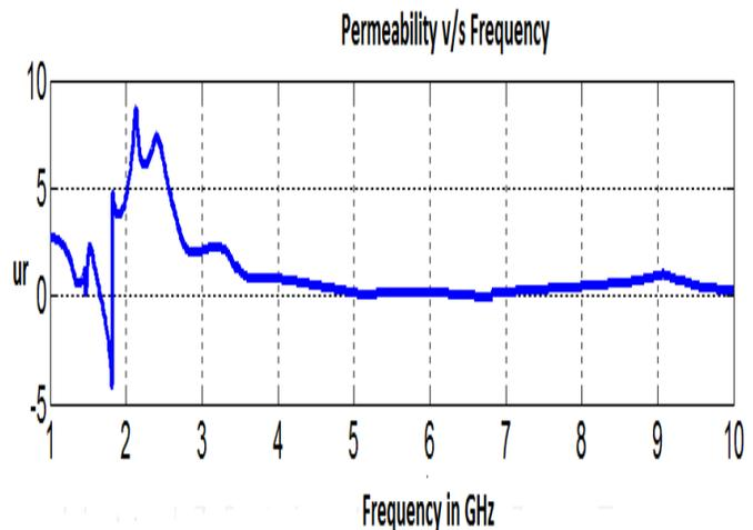
**Figure 7.** Retrieval results of 8-shaped DNG MTM for Permeability ( $\mu_r$ )
