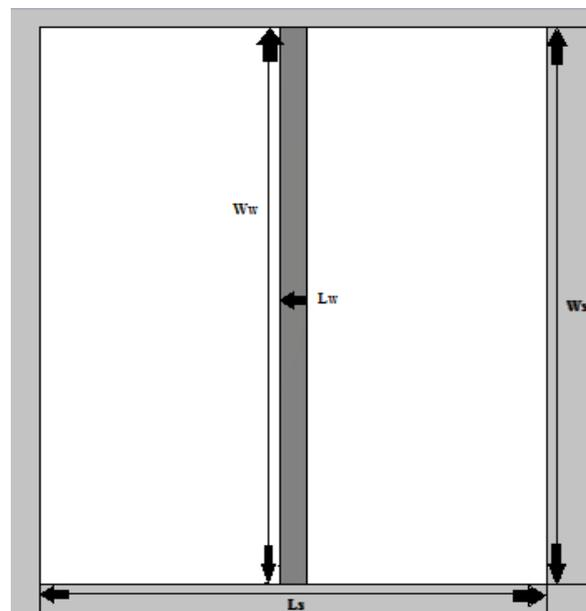
Figure 3 Back View of DNG Metamaterial
