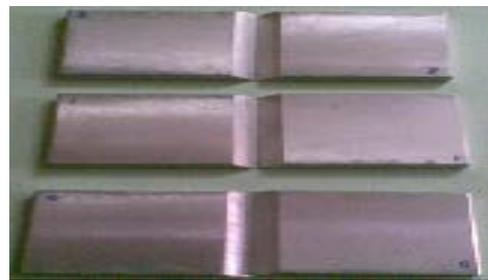
Figure 2 : Plates with edge preparation
