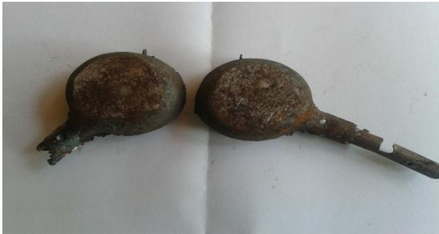
Figure 1. Liquid bath metal for open carbon testing
